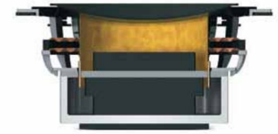
Conventional driver traps air inside
