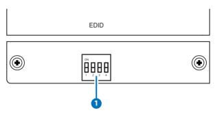
1 EDID: EDID switch offers EDID selection. There are 16 sets of EDID selection totally which divide to three modes includes "internal mode", "user mode" and "native mode". 6 set of internal EDID, 9 sets are defined as user mode which are allowing customer to
