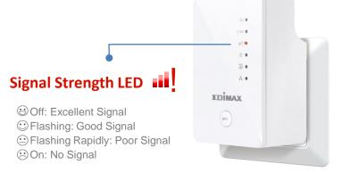
Install the extender where the signal strength LED is off (but not flashing) for optimal Wi-Fi performance.
