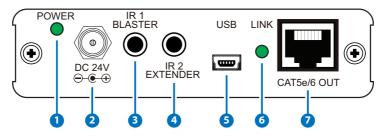
**1 POWER LED:** Once the power supply is connected the LED will illuminate.
