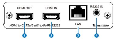
**1 HDMI OUT:** Connect to HDMI display for instant image display or cascade with another family type Transmitter. The unit will detect CAT5e/6/7 output's EDID when it obtain a 4Kx2K EDID and send out the signal accordingly to other output ports. If CAT5e/6/7 output is without a 4Kx2K's EDID the unit will detect all output's EDID and send out the signal that all outputs can accept.
