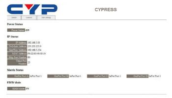
Click on the 'Control' tab to control power, input/output ports, EDID and reset mode.
