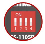
Switching all DIP switches to "ON" enables Surveillance-mode
