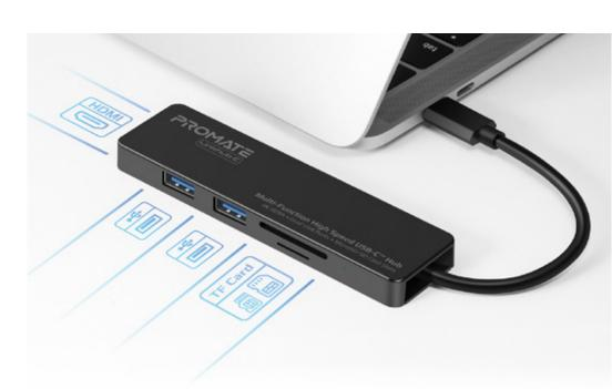
LinkHub-C adds 2 additional USB ports, 4K HDMI port and a MicroSD/SD card slot, allowing you to connect USB devices such as digital cameras, phones, external hard drives, flash drives, and printers all at one convenient place. The USB-A ports support a data transfer speed of up to 5Gbps. LinkHub-C does not require any software or complicated installation process, just plug it in and use.
