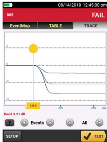
Bend as seen on an OTDR trace
